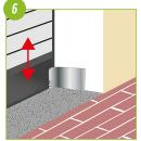
Check the position of the Skipper again by raising and lowering the door and adjust if necessary.
