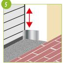
Using pliers, bend the cut-out lips to the shape of the door so that it seals properly.
