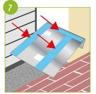
Remove the marked stickers and permanently fix the Skipper to the wall.
